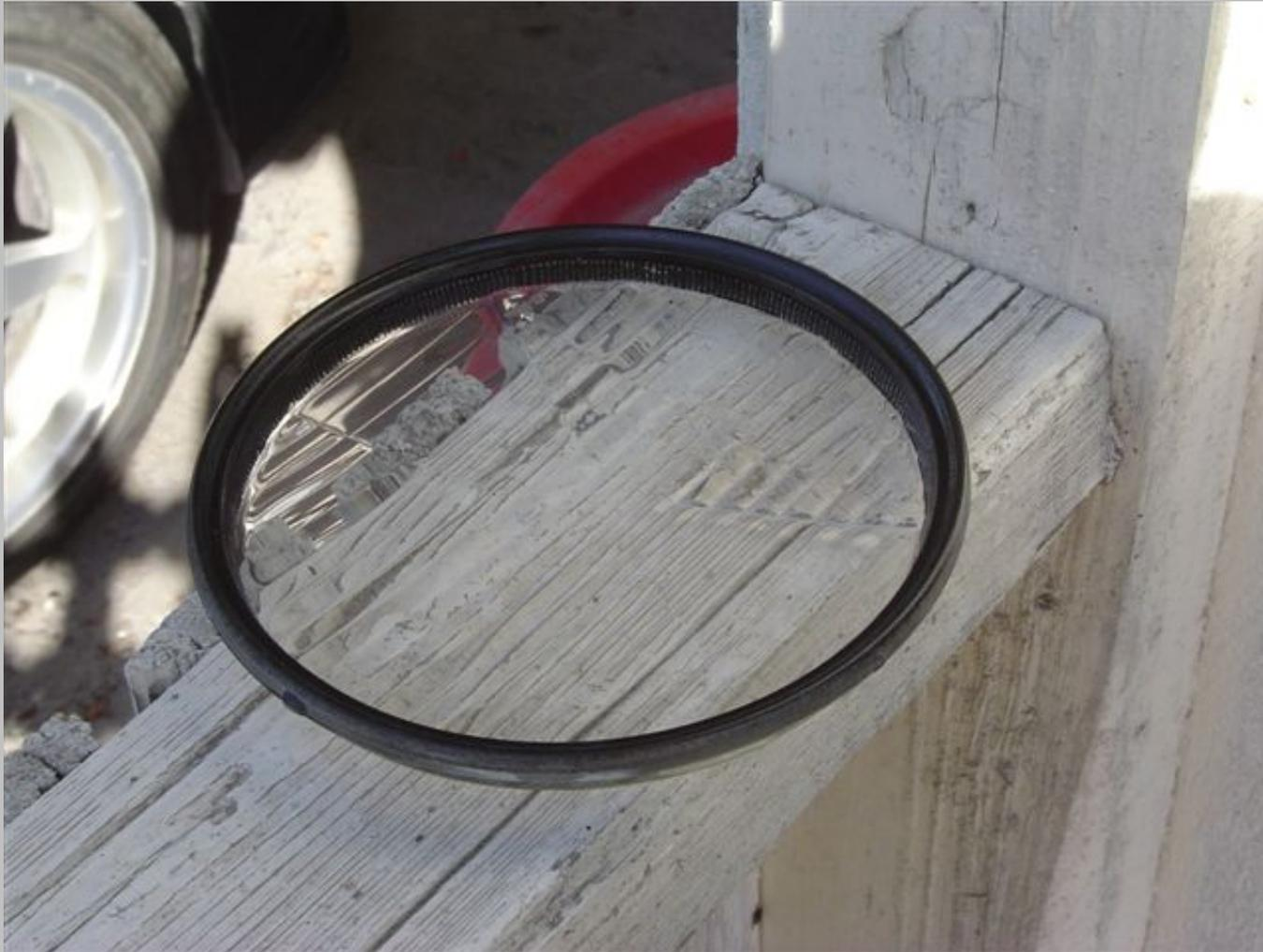
Then I coloured the shield inside the driving light projector unit black too, I painted a piece of galvanised steel and glued it to the shield facing out toward the magnifying glass, rather than try to spray it. It shows a little as you can see from the picture below left is coloured right is not.
